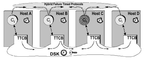
Figure 20 — Fail-controlled with a TTCB
