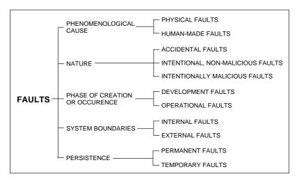
Figure 2 — Classes of elementary faults
